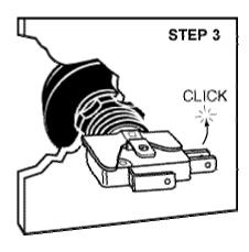
To remove, turn Switch-Lampholder to left and pull out.
