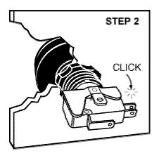
While applying slight pressure, turn Switch-Lampholder to right until it clicks into place.
