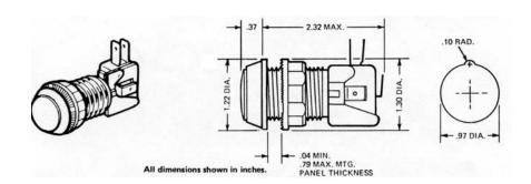
The X-6000 Illuminated Pushbutton is rugged, dependable and easy to install. Its durability has been proven in thousands of installations. The built in lamp serves to indicate which selection is playing in multiple button installations, as well as to indicate in use in single selection exhibits
